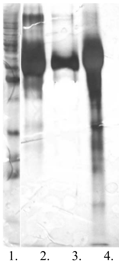
Fig. 3. SDS-PAGE in 12% polyacrylamide gel detected by silver: 1. standard; 2. urine proteins before albumin extraction; 3. supernatant containing albumin after centrifugation; 4. urine proteins after albumin extraction.
