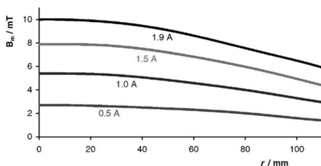
Fig. 1. Magnetic field distribution for magnetic field amplitude  $B_m$  inside the coil for different currents. Position  $r = 0$  mm denotes the centre of the coil.
