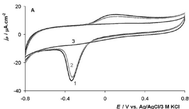
Fig. 2A. Cyclic voltammogram of living bacteria-covered glassy carbon electrode (bcGCE). Scan rate was adjusted to  $\nu = 50$  mV.s<sup>-1</sup>, 5<sup>th</sup> scans. Curve 1 – bcGCE in electrolyte (PBS). Two peaks (oxidation peak  $P_{\text{ox}}$  and reduction peak  $P_{\text{red}}$ ) can be observed. Curve 2 – system after 24 min at  $B_m = 10$  mT. Curve 3 – electrode covered with a layer of dead SRB.
