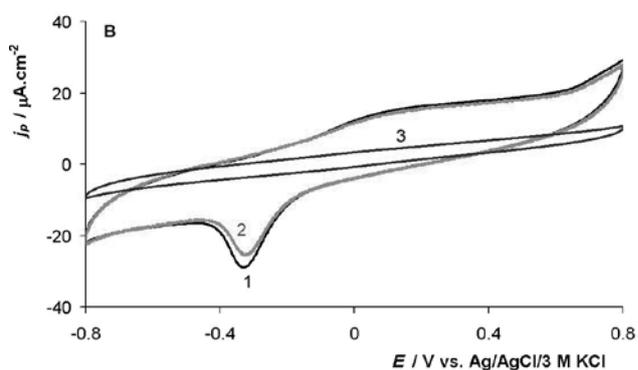
Fig. 2B. Cyclic voltammogram of living bacteria-covered pyrolytic carbon electrode in basal orientation (bcPGEb). Scan rate was adjusted to  $\nu = 50$  mV.s<sup>-1</sup>, 5<sup>th</sup> scans. Curve 1 – bcPGEb in electrolyte (PBS). Two peaks (oxidation peak  $P_{\text{ox}}$  and reduction peak  $P_{\text{red}}$ ) can be observed. Curve 2 – system after 24 min at  $B_m = 10$  mT. Curve 3 – electrode covered with a layer of dead SRB.
