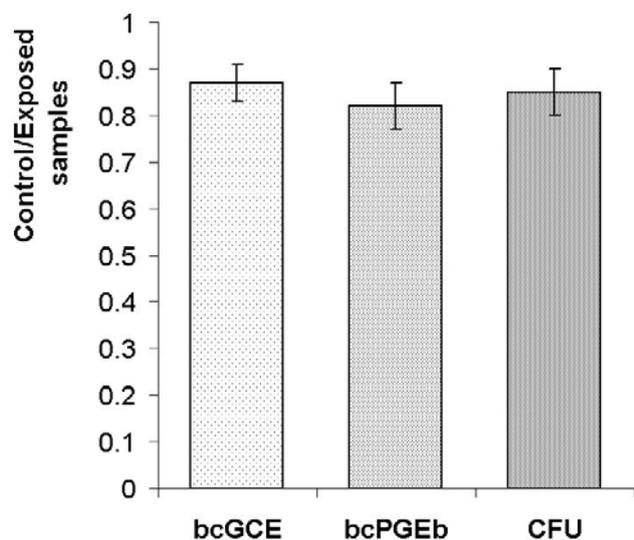
Fig. 3. Plot graph summarizing the effect of EMF ( $B_m = 10$  mT,  $f = 50$  Hz,  $t = 24$  min) on the SRB. Vertical axis represents the ratio control/exposed sample. This relative number denotes, in case of bcPGEb and bcGCE, the ratio between  $j_p$  (and thus effects of EMF on desulphurization activity of SRB) and in case of CFU the ratio between the CFU number of control/exposed sample (has a meaning of survived bacteria after magnetic field exposure).
